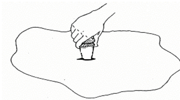
Figure 2. Wood Plug Installation.
